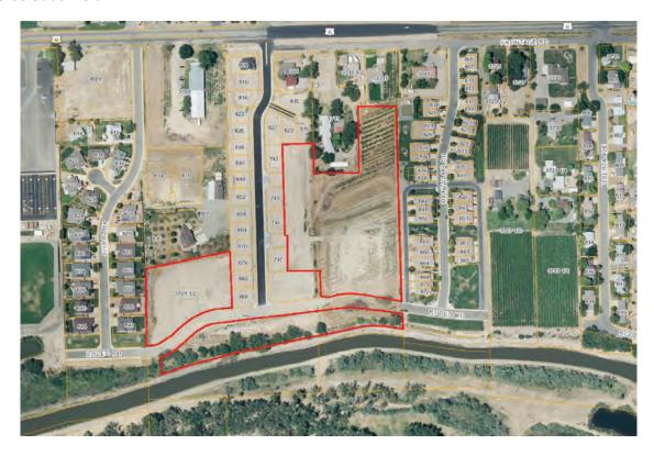
Rupp Avenue, constructed as part of Filing 1 improvements, provides access to Filing 2 from Hwy 6/G Road south to Fairhaven Road. Right-of-way for Fairhaven Road was dedicated to the Town of Palisade with Filing 1 improvements. Filing 2 is shown below as Lots 100, 101 and 102 on the plat below.
